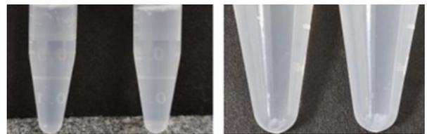
Figure 2b Appearance of 0.8 mg/mL paclitaxel nanocrystal formulation in dialysis bag at the end of release at 120 h (left) and after low-speed centrifugation (right)
