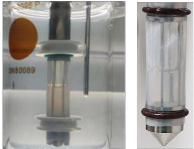
The dialysis membrane prevents the nanoparticles from entering the dissolution medium.
