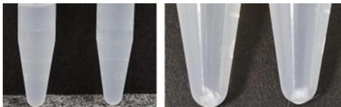
Figure 3b Appearance of 1.0 mg/ml PXT nanocrystal formulation in dialysis bag at end of release at 120 h (left) and after low-speed centrifugation (right)
