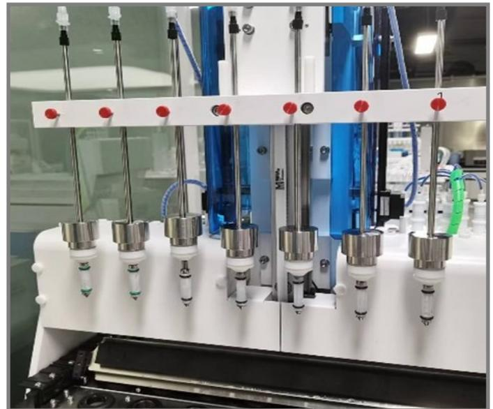
The mechanical reciprocating motion of the apparatus releases the nanoparticles into the medium through the membrane. The concentration of the drug in the release medium is sampled and measured at suitable time points.
