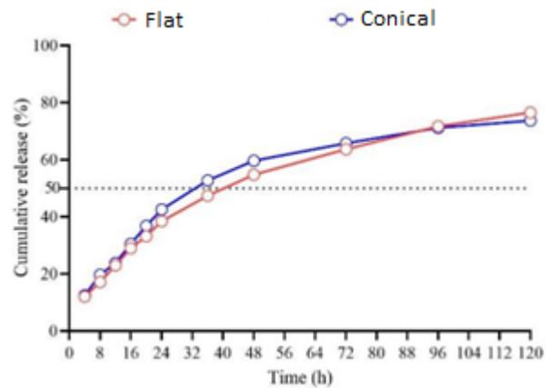
Figure 2a Cumulative release profile of 0.8 mg/ml paclitaxel nanocrystals in dialysis bags using flat or conical bottom frames.
