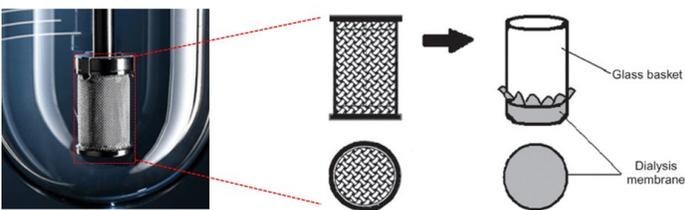
*"Closed bag" nanoparticle dissolution apparatus*
