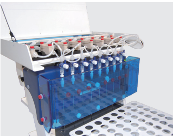
Cell holder system with 8 diffusion cells
