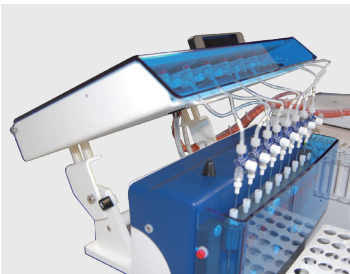
Cell holder lifted up to purge air bubbles
