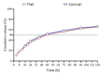
Figure 3a Cumulative release profile of 1.0 mg/ml paclitaxel nanocrystals in dialysis bags using flat or conical bottom frames.
