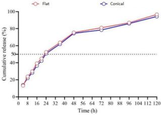
Figure 1a Cumulative release profile of 0.6 mg/ml paclitaxel nanocrystals in dialysis bags using flat or conical bottom frames.
