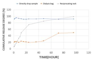
Graph shows significant differences between dissolution methods
