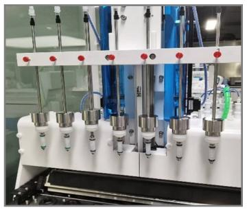
The mechanical reciprocating motion of the apparatus releases the nanoparticles int the medium though the membrane. The concentration of the drug in the release medium is sampled and measured at suitable time points.
